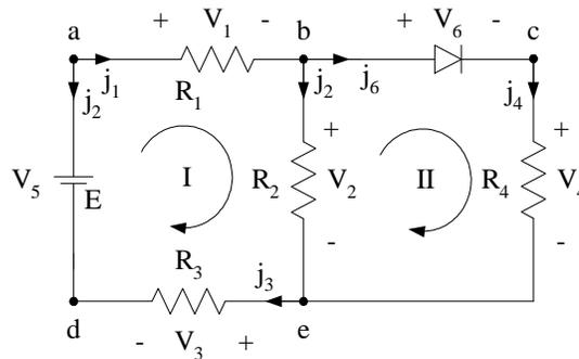
$$E = 10 \text{ V}, R_1 = R_4 = 22 \text{ k}\Omega \text{ y } R_2 = R_3 = 18 \text{ k}\Omega$$
