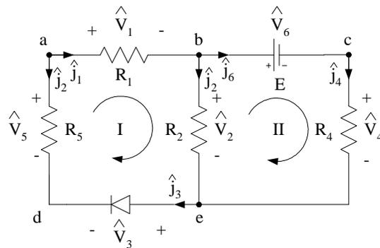
$$E = 10 \text{ V}, R_1 = R_5 = 18 \text{ k}\Omega \text{ y } R_2 = R_4 = 22 \text{ k}\Omega$$
